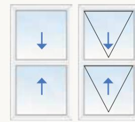
**Hinged:** Opening inwards, hinged units provide full access to the primary window. Single or double openers are available for both domestic and commercial sized windows. Hinged units are perfect for fire escapes and for French or Patio doors.
